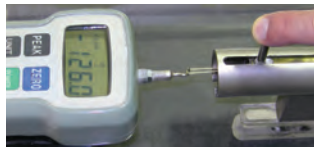
G&H® calibrated load cell testing regularly during production ensures exact and consistent force values. Elastics are tested at the industry standard expansion of 3 times passive diameter. Elastic samples are visually inspected and quality checked.
